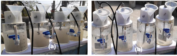
Fig. 4: The turbidity during test in Jar tester (a) with waste water and (b) after treatment.
